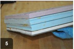
All XPS layers should be attached firmly to one another and square to hatch
