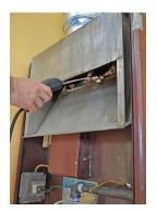
Test undiluted flue gases in natural draft furnaces
