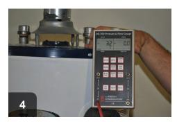
After mitigation, verify that depressurization limits are not being exceeded
