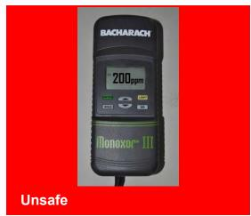
CO levels cannot exceed 200ppm as measured, unless to manufacturer specs
