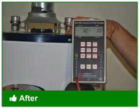
Test that depressurization limit is not being exceeded by new ventilation
