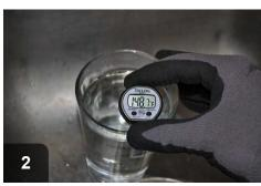
Hot water temperatures should not exceed 120 degrees Fahrenheit
