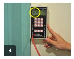
With hose under door, check pressure again. Readings >+/-3pa are no good and require interior ventilation
