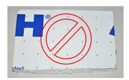
Do NOT use EPS in air returns due to proximity to combustion appliances
