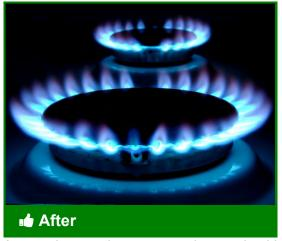
A properly operating gas range burner should have an even blue flame
