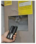
Complete spillage testing on all combustion appliances
