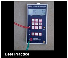
For DG700, Input and Reference hoses should be mounted to the same side
