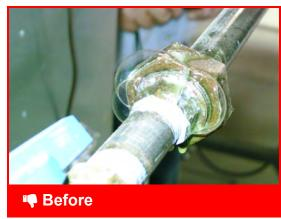
Fuel lines should be inspected for leakage
