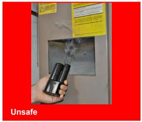
Conduct spillage and depressurization testing at the end of the work day
