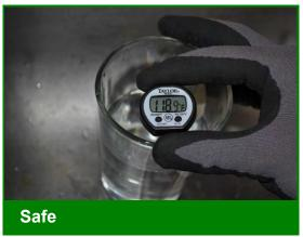
Water heaters should produce water under 120 degrees to prevent scalding
