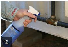
Use multiple methods to test for leakage--bubble solution
