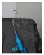
With blower door running, chemical smoke should not draw into test holes
