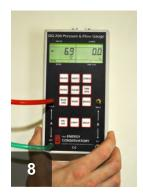
Manometer reading should not be more negative than allowable depressurization limit
