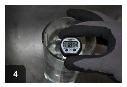
After adjustment and insulation, retest to verify temp is under 120 degrees
