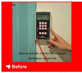
If reading is >+/-3pa, interior ventilation needs to be installed
