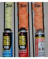
Spray foam can be used to span gaps up to 3 inches
