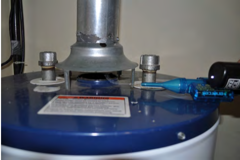
Complete spillage test using chemical smoke pencil
