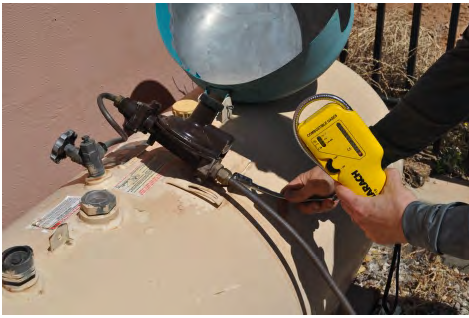
Check all raw fuel lines for leaks
