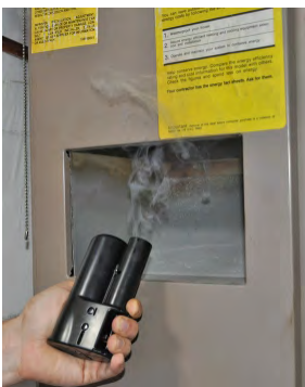
Complete spillage testing on all combustion appliances
