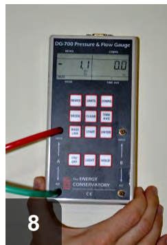
8 Conduct spillage and draft test under worst case CAZ depressurization
