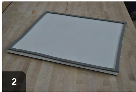
2 Ensure an air tight seal by making sure foam tape has no gaps
