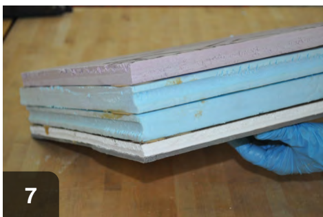
7 All XPS layers should be attached firmly to one another and square to hatch
