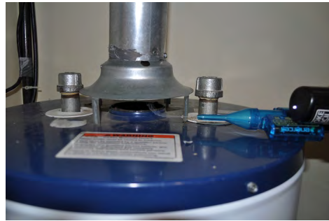
Complete spillage test using chemical smoke pencil
